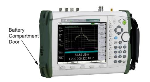
Figure 1-1. Battery Compartment Door
