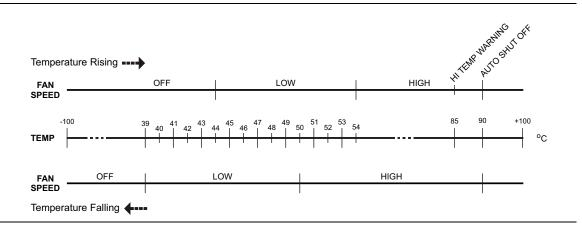
Figure B-1. Fan Speed versus Temperature
