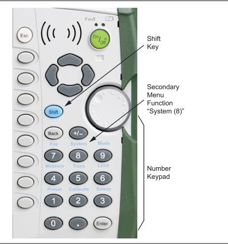
Figure 2-5. Keypad and Secondary Function Menus
