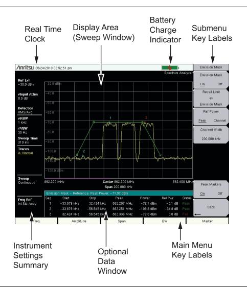
Figure 2-6. Spectrum Analyzer Display
